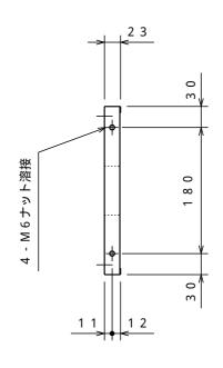
棚板:SPCC-SD t0.7 補強:SPCC-SD t0.7
